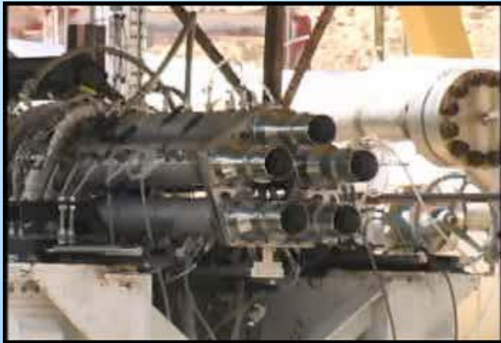
Test firing of five tube PDE
