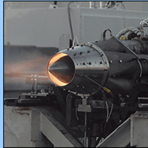
Five tube PDE fitted with compound nozzle.
